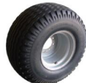
A agricultural wheel 500/50-17 14 plies Width 20 in Diameter 37 in
